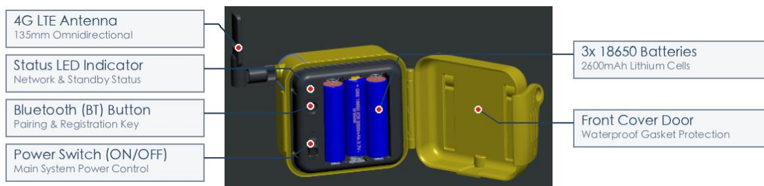
Figure 2.2: Camera Open Internal View Photo Diagram (Status LED, BT Button, Power Switch & Battery Compartment)
